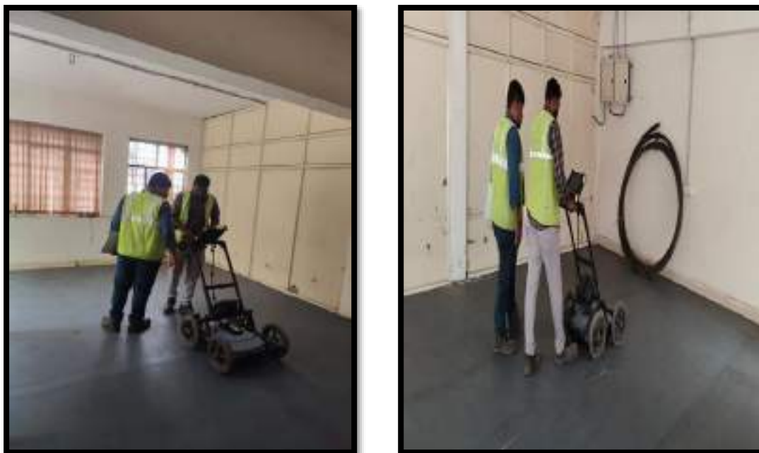
Figure 7.7: GPR survey for determining the depth and size of footing
