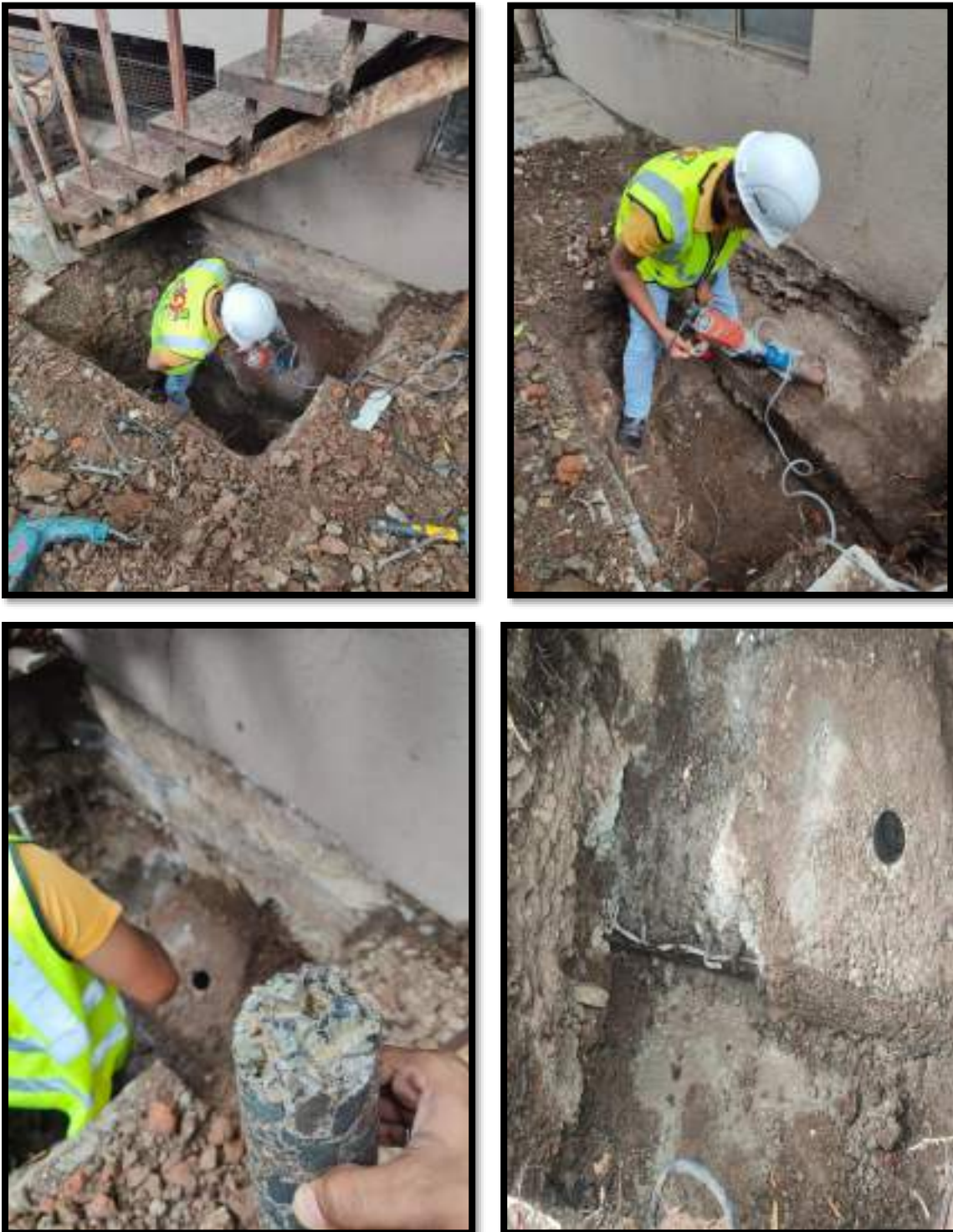
Figure 7.3: Execution of core test for determination of compressive strength of the footing
