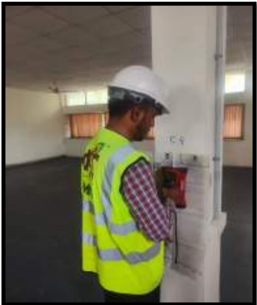
Figure 7.4: Execution of rebar scanning for detection of reinforcement and concrete cover in the structural elements
