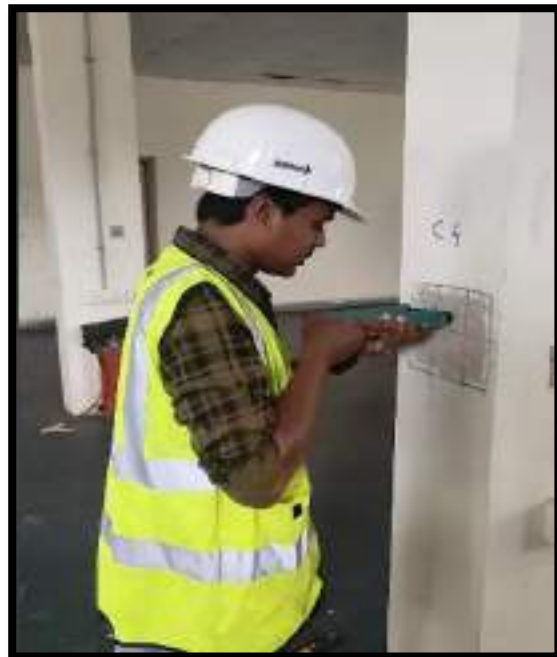
Figure 7.1: Execution of rebound hammer test to determine the approximate compressive strength of the column
