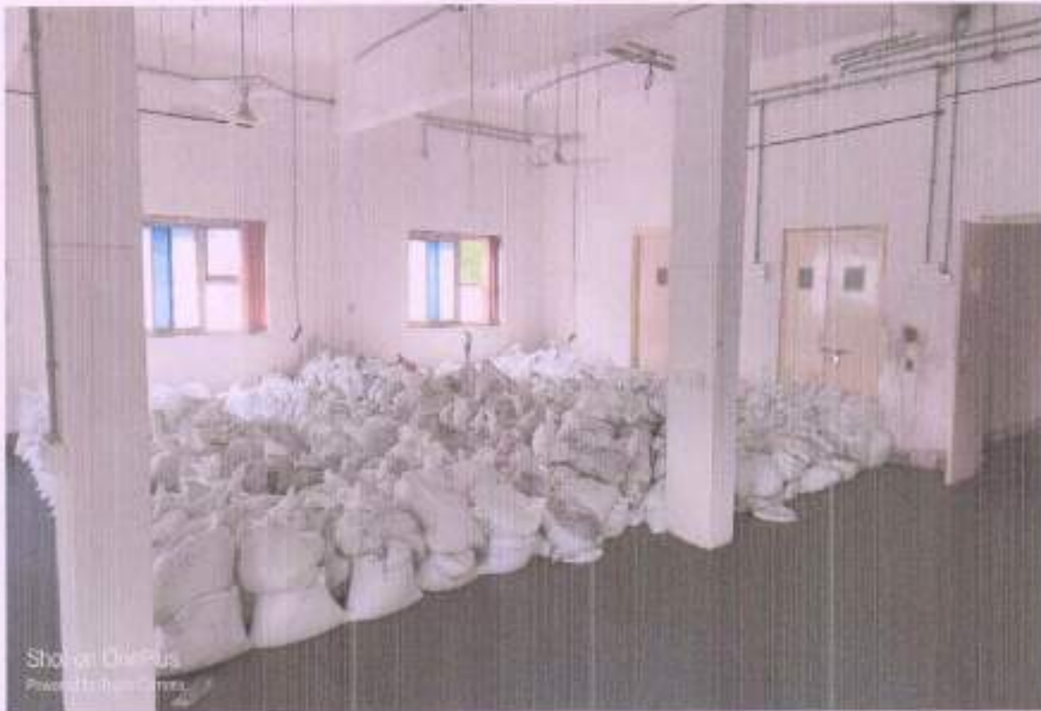
Photo 2: View of loading [ 4.5 \times 1.25 = 5.31 \text{ kN/m}^2 ] on RC slab of Jidnyasa Building, NCCS, Pune.
