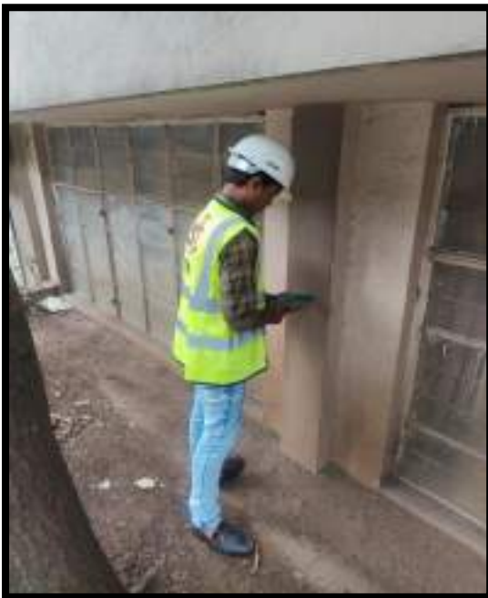
Figure 7.1: Execution of rebound hammer test to determine the approximate compressive strength of the column
