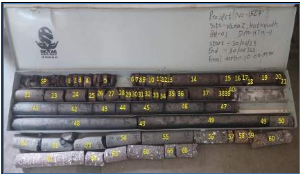
Figure 7.5: Drilling for taking out samples for checking safe bearing capacity of soil
