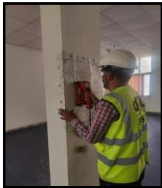
Figure 7.4: Execution of rebar scanning for detection of reinforcement and concrete cover in the structural elements
