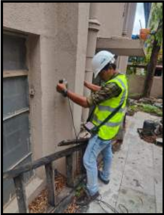
Figure 7.2: The ultrasonic pulse velocity test shows that the distance between the transducer and receiver divided by time gives velocity of the wave of propagation in concrete.
