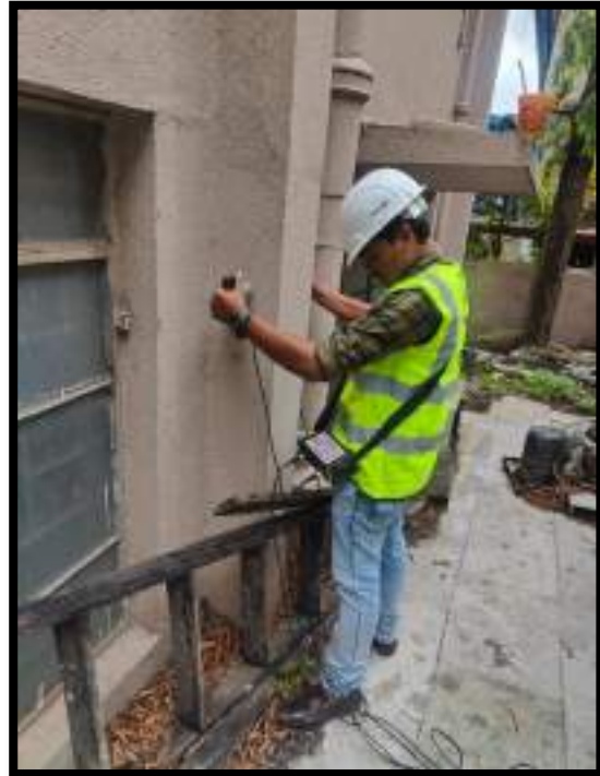
Figure 7.2: The ultrasonic pulse velocity test shows that the distance between the transducer and receiver divided by time gives velocity of the wave of propagation in concrete.
